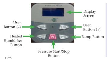
To enter the Clinician's Set-Up Menu, remove the power cord from the rear of the RESmartTM unit. Press and hold both the start and ramp buttons simultaneously, while reconnecting the power cord. The RESmart TM unit may now be programmed with the therapy options.
